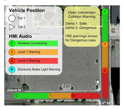
Prior to the warnings, the availability of reliable wireless connectivity is highlighted in green. Note that the Cohda Radio established a robust link well before any potential danger, allowing the safety system maximum opportunity to take action.
