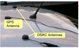
The ST Cartesio Processor includes a high quality embedded GPS receiver to provide current location and time. This information is used to build SAE J2735 Basic Safety Messages, which are then broadcast via the Cohda 802.11p Radio, at a rate of 10 messages per second.
